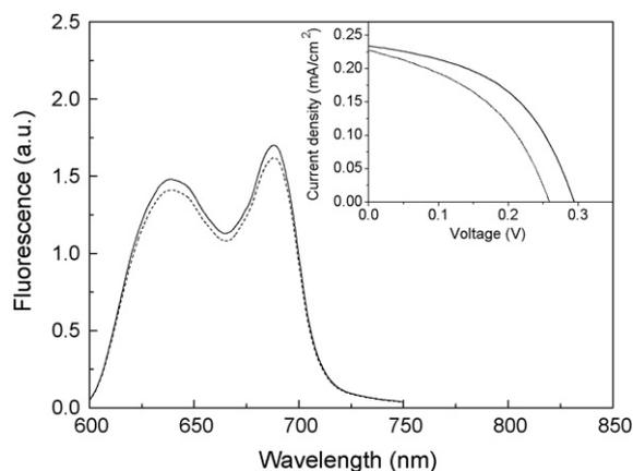
**Fig. 5.** Fluorescence spectra of the dye Ru470 sensitized nanocrystalline  $\text{TiO}_2$  films after solar cell measurements in a different electrolyte. The inset: the corresponding photocurrent–voltage curves of the DSSCs. The standard electrolyte: dashed line; the  $\text{Li}_2\text{CO}_3$  saturated electrolyte: solid line. The excitation wavelength for fluorescence was 480 nm.
