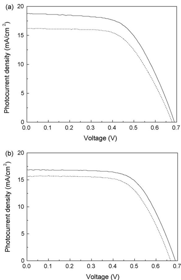
Fig. 2. Photocurrent–voltage characteristics of the DSSCs which compare the effect of the standard electrolyte with  $\text{Li}_2\text{CO}_3$  (a) and  $\text{K}_2\text{CO}_3$  (b). The standard electrolyte: dashed line; the electrolyte with additions: solid line.
