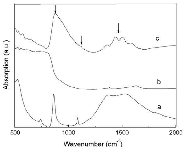
**Fig. 4.** FT-IR spectra of pure  $\text{Li}_2\text{CO}_3$  (a) and  $\text{TiO}_2$  (b) and  $\text{TiO}_2$  coated with  $\text{Li}_2\text{CO}_3$  (c). For pure  $\text{Li}_2\text{CO}_3$  and  $\text{TiO}_2$ , KBr disk as background; for  $\text{TiO}_2$  coated with  $\text{Li}_2\text{CO}_3$ , the mixture of 195 mg KBr and 5 mg  $\text{TiO}_2$  as background. The arrow indicates the IR peak position corresponding to  $\text{Li}_2\text{CO}_3$ .
