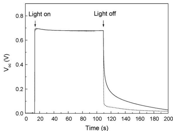
**Fig. 6.**  $V_{oc}$  decay curves with time for the DSSCs based on a different electrolyte. The  $V_{oc}$  of the standard DSSC (dotted line) was normalized to that of the DSSC based on the  $\text{Li}_2\text{CO}_3$  saturated electrolyte (solid line).
