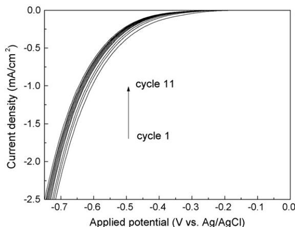
Fig. 3. A series of current–voltage curves of the nanocrystalline  $\text{TiO}_2$  thin film cell with the  $\text{CO}_2$  electrolyte in the dark. Scan rates: 5  $\text{mV}/\text{s}$ .
