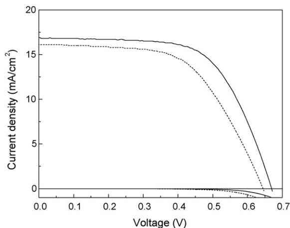
**Fig. 1.** Current–voltage characteristics of the DSSC which differ by the electrolyte under illumination and in the dark. The standard electrolyte: dashed line; the  $\text{CO}_2$  electrolyte: solid line.
