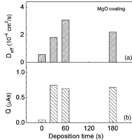
FIG. 6. Dependence of the effective diffusion coefficient (a) and the integrated charge (b) on the deposition time of the MgO coating layer, i.e., its thickness.
