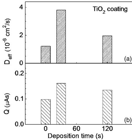
FIG. 5. Dependence of the effective diffusion coefficient (a) and the integrated charge (b) on the deposition time of the TiO<sub>2</sub> coating layer, i.e., its thickness.
