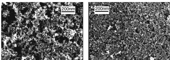
FIG. 3. Micrographs of the top views of unpressed porous TiO<sub>2</sub> layer deposited by EPD (a) and of a nanoporous TiO<sub>2</sub> layer after pressing (b).
