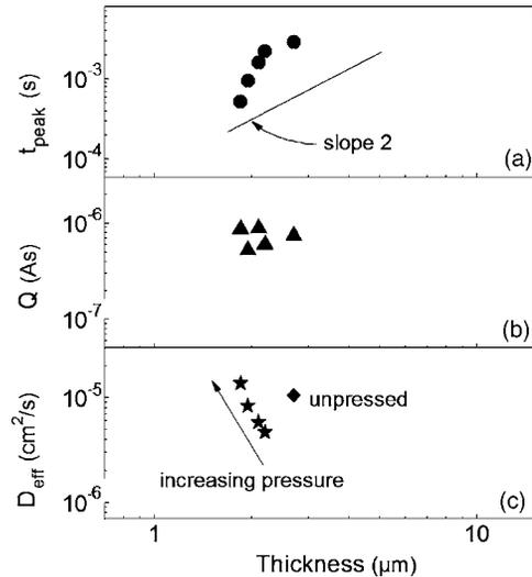
FIG. 4. Thickness dependence of the peak time (a), the integrated charge (b), and the effective diffusion coefficient (c) for the unpressed and pressed with different pressures nanoporous TiO<sub>2</sub> layers. The line in (a) represents a slope of 2. Note the increase of the effective diffusion coefficient with increasing pressure of the pressed nanoporous TiO<sub>2</sub> layers (c).
