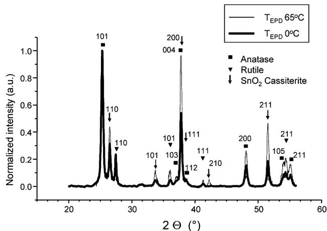
**Figure 2.** XRD profiles of films prepared using EPD under 0 and 65 °C.
