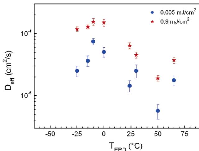
**Figure 5.** Temperature dependent on the effective diffusion coefficient calculated from transients that were excited using laser energy of  $0.005$  mJ/cm<sup>2</sup> (circles) and  $0.9$  mJ/cm<sup>2</sup> (stars).
