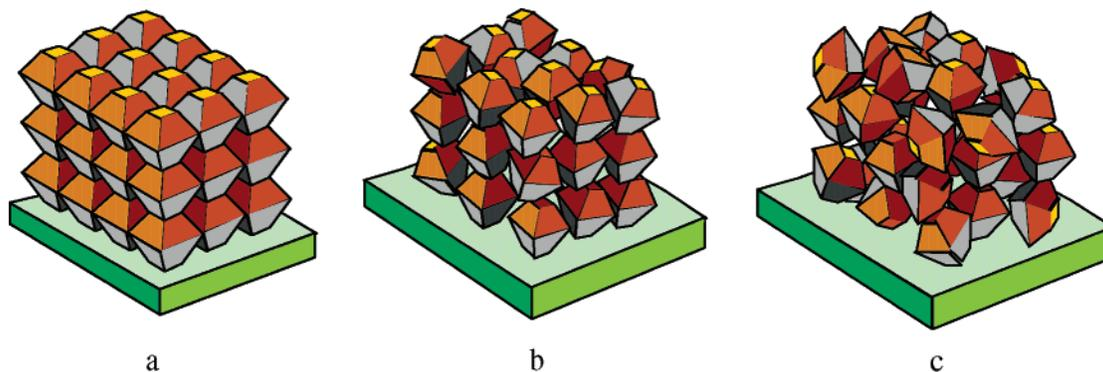
**Figure 1.** Anatase TiO<sub>2</sub> nanoparticles with their truncated polygon crystal habit, packed in three main possibilities in a nanoporous layer: (a) perfectly oriented nanoparticles; (b) partially oriented nanoparticles; (c) randomly oriented nanoparticles.
