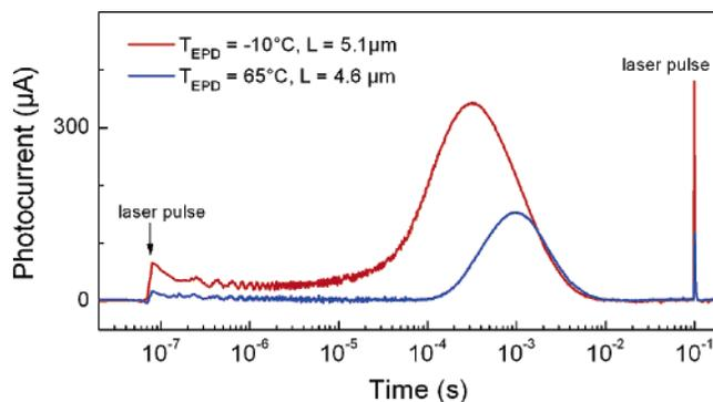
**Figure 4.** Photocurrent transients profiles of transients passed through nanoporous films prepared by EPD under  $-10$  and  $+65$  °C. (Transients executed using a laser excitation energy of  $0.9$  mJ/cm<sup>2</sup>.)
