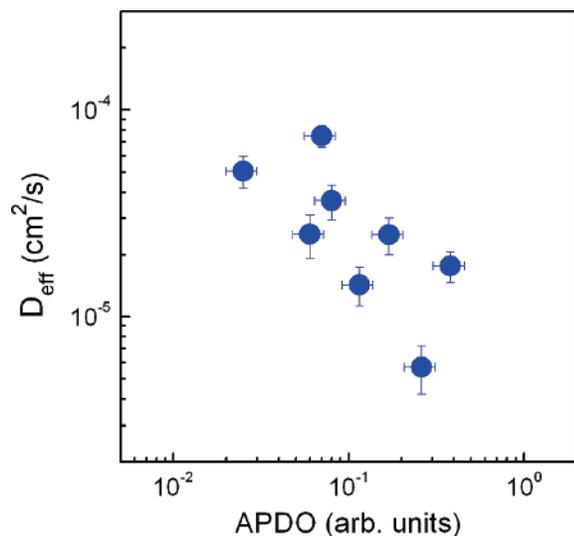
**Figure 6.** Effective diffusion coefficient dependent on the average degree of preferred orientation (ADPO) in anatase nanoparticles (transients executed using laser excitation energy of 0.9 mJ/cm<sup>2</sup>).
