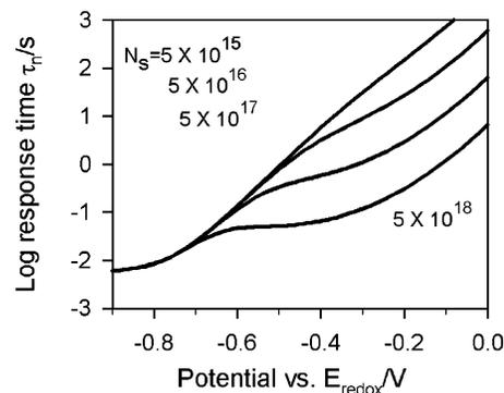
**Figure 3.** Representation of the response time in a DSSC as a function of open-circuit voltage. The DSSC simulation parameters are the same as those in Figure 2, and the surface trap density is varied as indicated in  $\text{cm}^{-3}$ .
