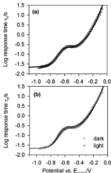
**Figure 6.** (a) Decay of the cell potential in a dye-sensitized solar cell with TBAI electrolyte following application of a negative bias ( $> -1.2$  V) in the dark. (b) Comparison of the photovoltage decay (light) and the decay of the potential following an applied bias (dark). Lines correspond to the fits to the model discussed in the text. Parameters are given in columns 1 and 2 of Table 1.
