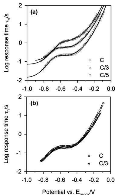
**Figure 7.** (a) Photovoltage decays of a single dye-sensitized solar cell with different concentrations of I<sub>3</sub><sup>-</sup>, changing in the proportion indicated, with  $c = 0.05$  M. Lines correspond to the fits to the model discussed in the text. Parameters are given in columns 3 to 5 of Table 1. (b) Rescaling of the data after dividing by 3 the data of  $\tau_n$  for  $c/3$ .
