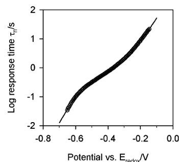
**Figure 8.** Comparison of the model results (thin line) with the measurement reported previously<sup>6</sup> of the response time in a DSSC with  $\text{Li}^+$  cation by open-circuit photovoltage decay.
