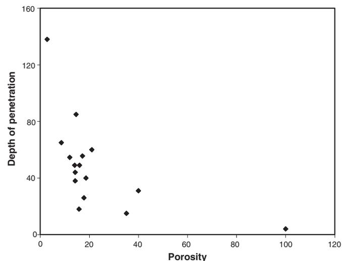
FIG. 5—Depth of fingerprint penetration (DFO, microns) vs. paper porosity (sec/100 cm<sup>3</sup>) for 13 uncoated papers.
