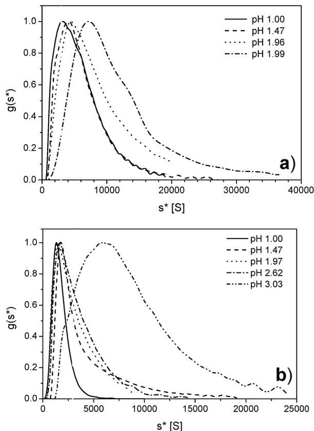
**Figure 4.** pH-dependent sedimentation coefficient distributions for (a) sample 2 and (b) sample 1.
