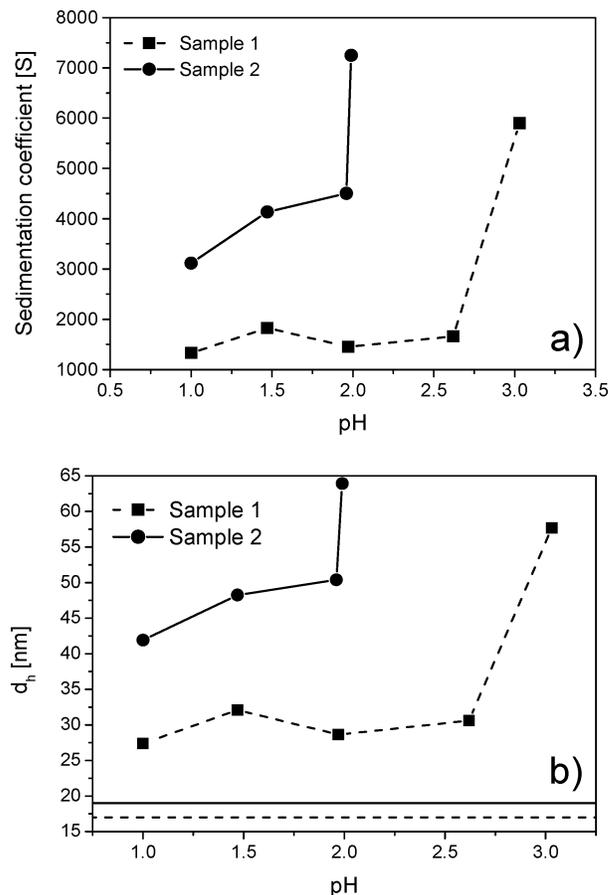
**Figure 5.** (a) Sedimentation coefficients from the peak maximum of the sedimentation coefficient distribution at different solution pHs; (b) pH-dependent particle sizes calculated on the basis of the sedimentation coefficients presented in part a with a bulk anatase density of 3.84 g/mL. The horizontal lines in part b indicate the particle diameters from electron microscopy and XRD (see above).
