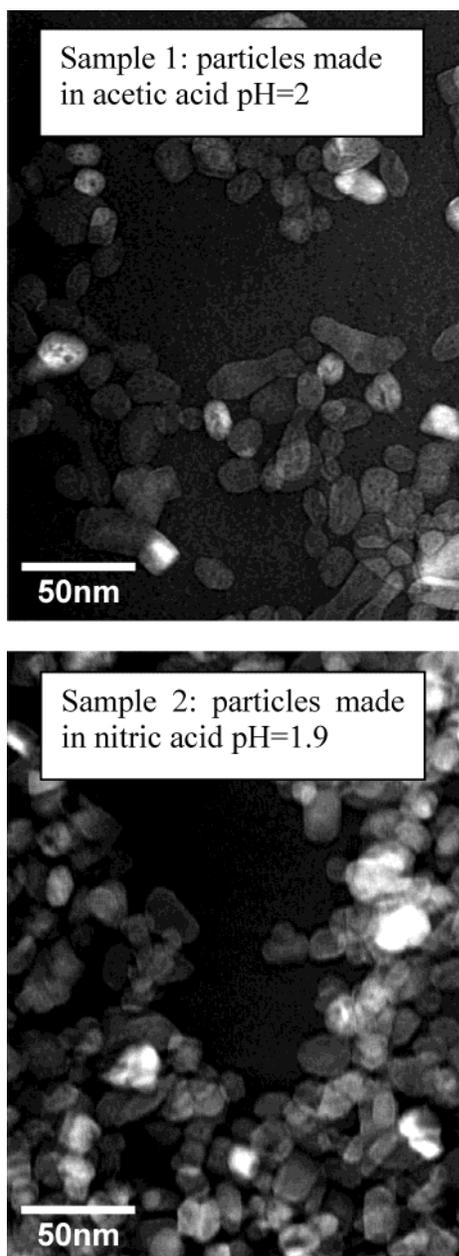
**Figure 1.** TEM pictures of the two nanosize  $\text{TiO}_2$  samples compared in this work showing an average crystallite size of 18.7 nm (standard deviation, 6.5) for sample 1 and 17.2 nm (standard deviation, 4.2) for sample 2.
