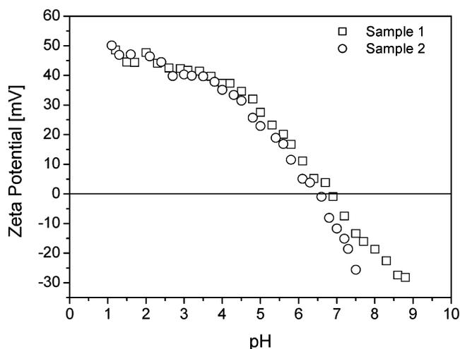
**Figure 3.** pH dependence of the  $\zeta$ -potential for samples 1 and 2.
