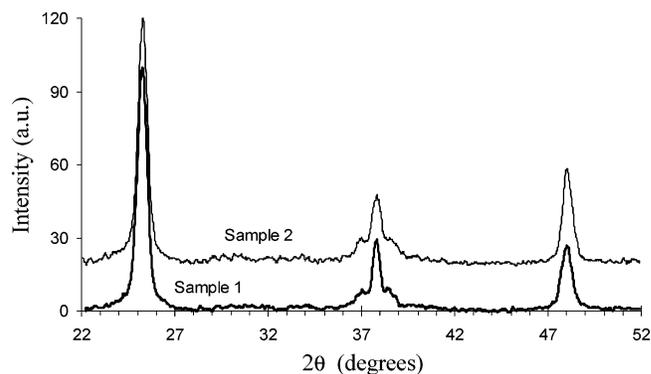
**Figure 2.** X-ray diffractograms of the two samples compared in this work indicating that both samples consist of anatase crystals. Volume-average grain sizes of 18.7 nm for sample 1 and 16.7 nm for sample 2 were calculated from the peak broadening of the diffractograms.
