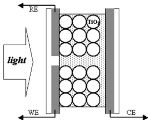
**Figure 2.** Schematic presentation of the 3-electrode DSSC. The standard 2-electrode measurement is performed using the working (sensitized) and counter electrodes. For a 3-electrode measurement of the same cell, the reference electrode maintaining  $V_{oc}$  is added.
