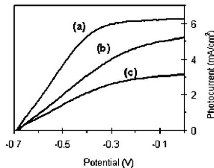
**Figure 5.** Three *iV* curves measured in a 3-electrode configuration using the same sensitized electrode and different counters. The different photocurrents obtained at similar applied voltages are attributed to recombination processes resulting from the counter electrode quality.
