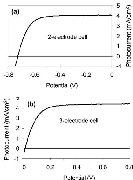
**Figure 3.** *iV* curves of (a) the 2-electrode and (b) the 3-electrode DSSC. The potentials are measured versus the counter electrode potential in the 2-electrode configuration, and versus the open circuit potential ( $V_{oc}$ ) in the 3-electrode setup. Note that the potential scales are shifted by the  $V_{oc}$  value.
