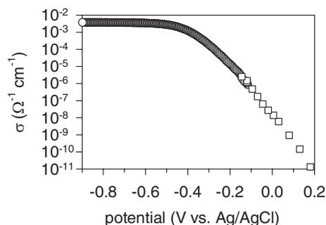
**Fig. 3** Electronic conductivity in nanostructured TiO<sub>2</sub> electrodes in solution at pH 2 as a function of the electrode potential. The square points were determined by EIS as indicated in Fig. 1. The circle points were determined in a coplanar configuration as indicated in Fig. 2. The EIS data have been shifted +80 mV to account for the difference of the activity of solutions used in the two measurements.
