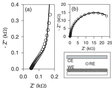
**Fig. 1** Experimental setup for measuring the electrochemical impedance and typical impedance spectrum of a nanostructured  $\text{TiO}_2$  film. a) High frequency data. b) Low frequency data. Dots are experimental data and lines are the fit of the transmission line model of Ref. [4].
