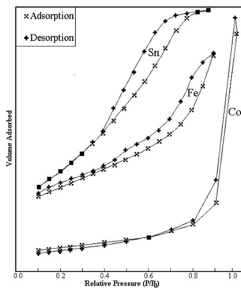
Fig. 4 Adsorption–desorption isotherm for mesoporous  $\text{SnO}_2$ , mesoporous  $\text{Fe}_2\text{O}_3$ , and porous  $\text{Co}_3\text{O}_4$ .
