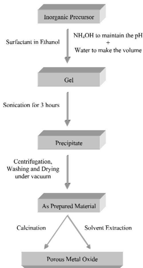
**Fig. 1** Schematic presentation of the method of preparation of porous metal oxide by sonochemical technique.
